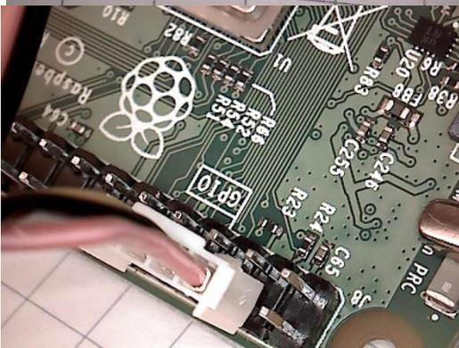
Unfortunately, the grid spacing of the connector strip and the GPS unit connector is different, but with a little bit of bending, a proper contact is achieved.
