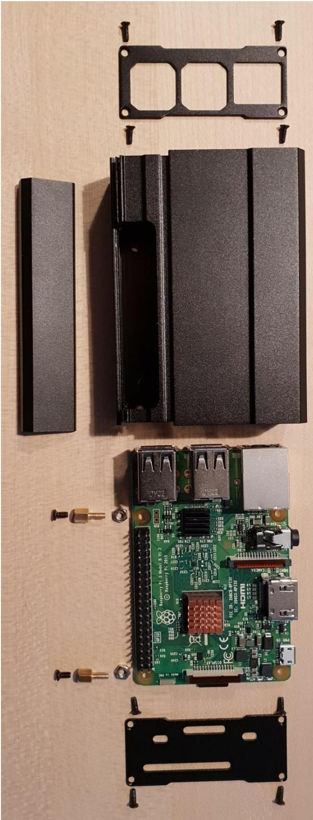
The upper face is screwed to the housing with 4 cross-head screws. (Thick edge to the bottom of the housing.)
