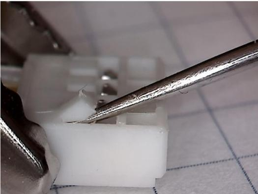
Lift the plastic spring with a pin and then pull out the black and the red wire. (See picture).
