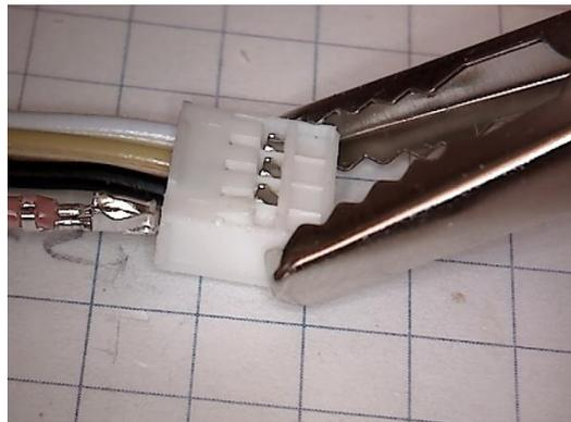
Then insert the two metal contacts (swapped over) back into the corresponding holes of the plastic plug. (see picture).
