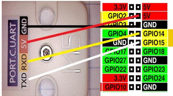
Unfortunately the supply lines (5V,GND) of the GPS unit must be crossed to match the pin assignment of the Raspi:
